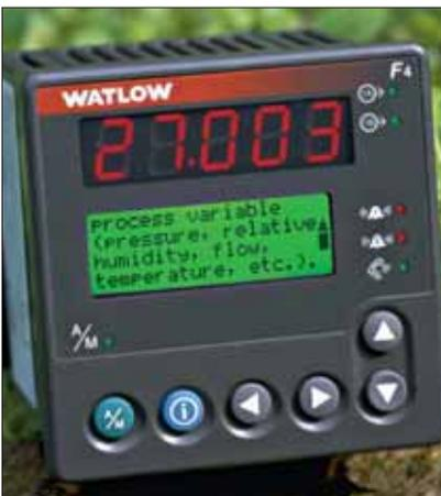
Available in  $\frac{1}{32}$ ,  $\frac{1}{16}$ ,  $\frac{1}{8}$  and  $\frac{1}{4}$  DIN sizes, agency approved Watlow single-loop, auto-tuning temperature controllers automatically set PID control parameters for optimum system performance. Manual settings also permit on-off, P, PI or PID control modes. All Watlow auto-tuning controllers are designed and manufactured to withstand harsh industrial environments and come with a three-year warranty for Control Confidence®.
