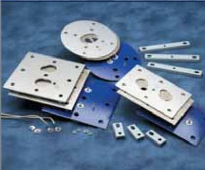
Watlow layers thick film resistor and dielectric materials on quartz, stainless steel and ceramic substrates to produce high performance industrial heaters. The thick film heaters provide very fast temperature response and fine thermal uniformity on a low-profile heater. Thick film heaters are ideal for applications where space is limited, where conventional heaters can't be used, when heat output needs vary across the surface, or in ultra-clean or aggressive chemical applications.
